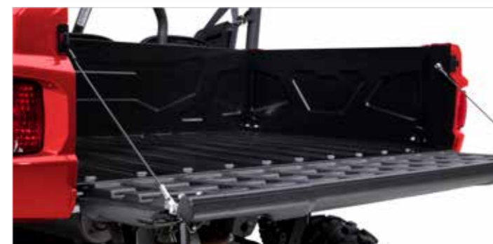
The rear load bed has an assisted tip-up plus a full width hinged rear access tail gate that can accommodate a Euro-pallet and 272kg in weight
