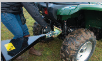
Swivel hitch and floating drawbar - light and safe
